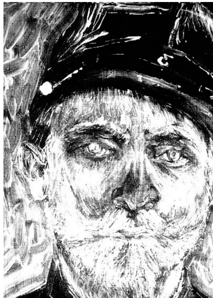
X-ray photograph of a Van Gogh painting, presumably a self-portrait, on canvas. X-rays are made to prove a paintings authenticity, check the condition of the canvas material, or determine possible paint-overs. Cadmium and/or lead in the paint absorb radiation, thus forming an image. Applied X-ray process data: 30 kV, 10 mA.min, Agfa D4 without lead screens and a source-to-film distance of 100 cm.
