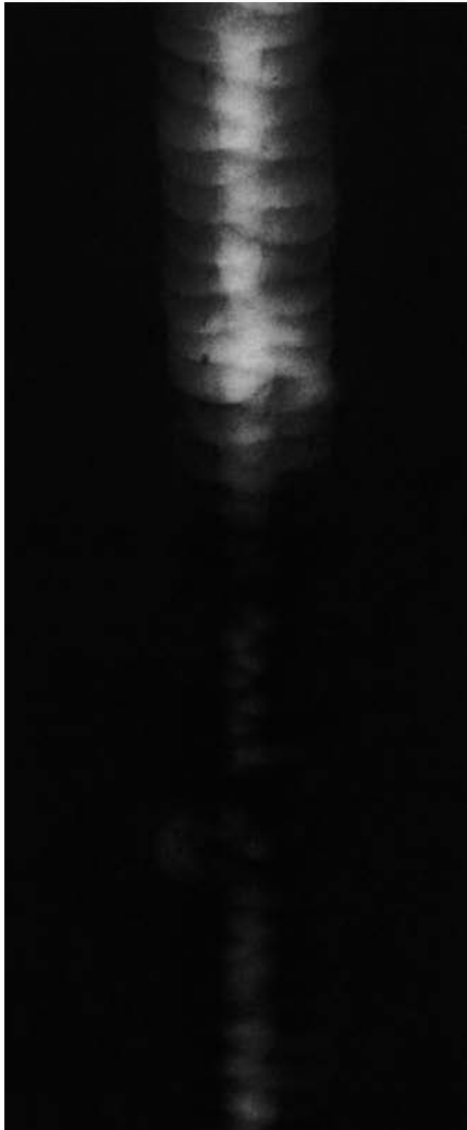
External concavity or insufficient fill. The weld density is darker than the density of the pieces welded and extending across the full width of the weld.
