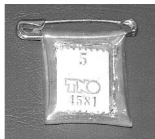
Fig. 4-19. Film dosimeter (film badge)
