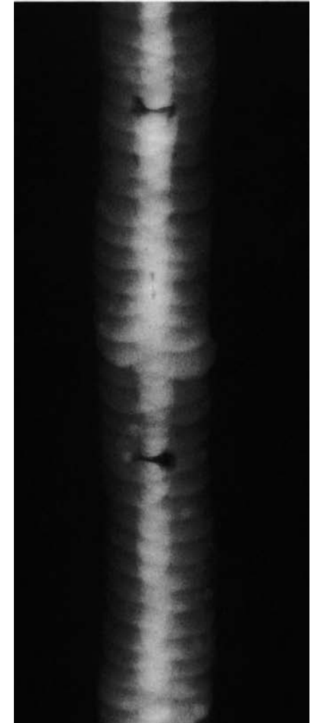
Interpass slag inclusions. Irregularly-shaped darker density spot, usually slightly elongated and randomly spaced.
