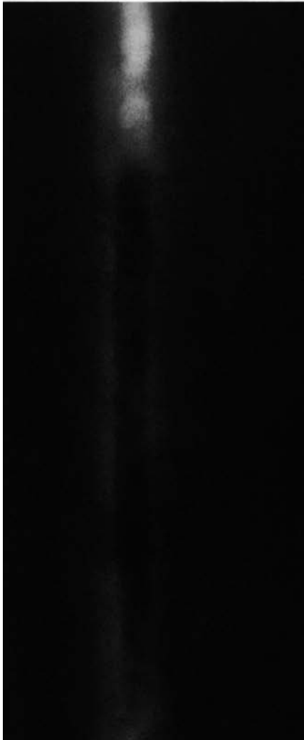
Internal concavity (suck back). An elongated irregular darker density with fuzzy edges, in the centre of the width of the weld image.
